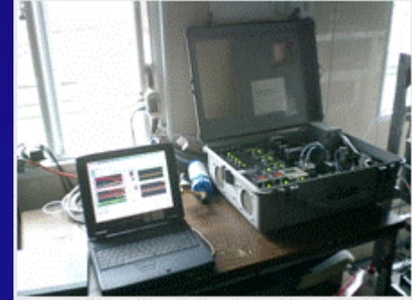
Fast olefin sensor (FOS) in EC mode (Hills Scientific Fast Isoprene Sensor)
